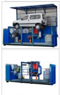
The depollution time was established on the basis of the compressed-air procedure offered including some 10 minutes setup time. On the basis of 8 hours running time daily, the system is capable of depolluting about 48 cars per day. The depollution technology has been developed by STH-Huber Anlagenbau GmbH, Germany. All types use the same depollution technology. The size of the carrier structure is 6500 x 2500 x 2500 mm (LxWxH).
