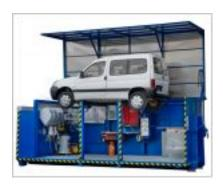
The STH-003/E/12/H mobile car depollution system is  $5400 \times 2200 \times 2200 \text{ mm}$  LxWxH in size with a maximum permissible load of  $5.0 \times 500 \times 1000$  (options).
